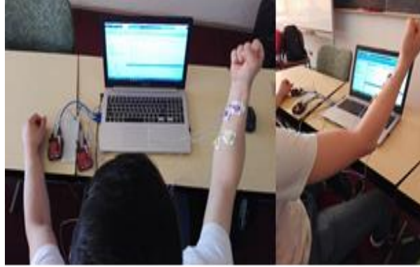
Fig. 1. 3-electrode EMG sensors position (MID -yellow, END -violet, GND in blue)
